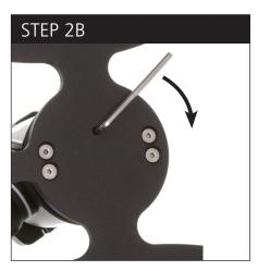
2B. Turn the low pod upside down and insert the 1/8" hex wrench into the lock screw access hole on the bottom of the low pod as shown in photo #2A and #2B. Tighten screw until slight resistance is felt.
