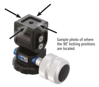
2. When the knob is loosened, the quick release will rotate 360 degrees with positive locking positions every 90 degrees as shown in photo 2.
