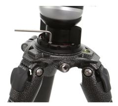
**2.** After you install the leveling base on your tripod, insert the 1/4-20 locking screw into one of the 3 threaded holes in the leveling base and use enclosed hex wrench to securely tighten the screw. The hex wrench and screw are enclosed in the packet with the red label.
