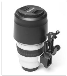
7. The LS-1 lens support can be removed and installed on the bottom dovetail, allowing the lens hood to be reversed for storage. Note: The stop on the LS-1 must fall inside one of the cavities in the lens foot.
