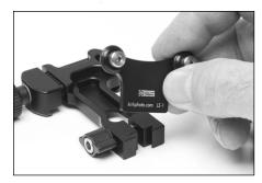
1. Insert roller bearing support into the quick release lens bracket with the writing facing outward. The quick release should be facing down.
