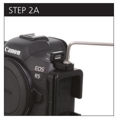
Take the enclosed camera strap connector (d) and the camera strap connector screw (e) and fully tighten with the 1/8 hex wrench (b) into place as shown in photo 2a and 2b.
