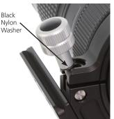
**6.** Again squeeze on the collar side and at the same time flip the knob back up to the locking position in the collar. Please note, while flipping the knob back into the locking position, make sure the black nylon washer is as shown in photo **6B** is positioned against the knob. After the knob is properly in position, you are now able to tighten and loosen the collar knob as needed.
